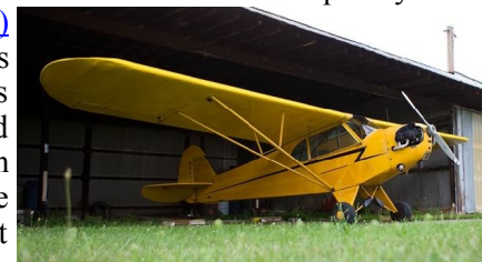
A Piper Cub is one example of an aircraft certificated without an electrical system.
